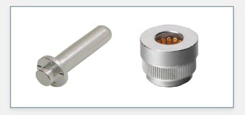
A reliable method to build connections between highpower busbars and boards in charging applications, the Sentrality Pin and Socket Interconnect System was designed with a +/- 1.00mm radial self-alignment to overcome tolerance stack-up issues.
